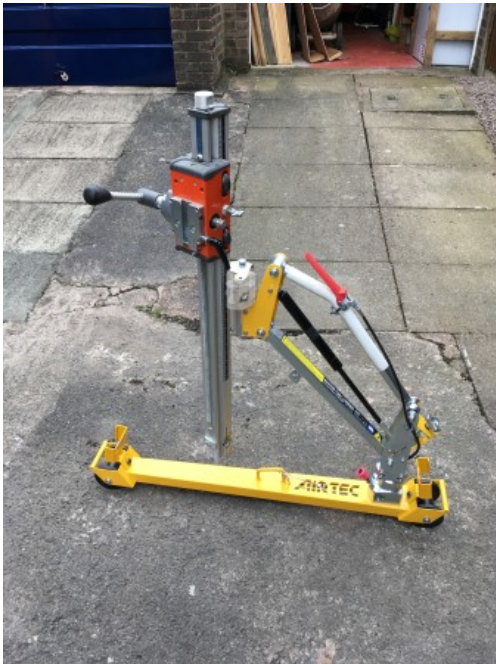
Master 35® tool carrier with core drilling machine
