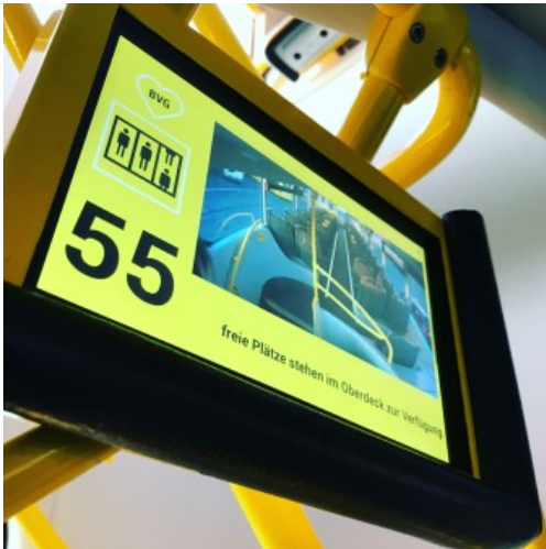
Upper deck – Display of fullness level for the BVG, Berlin's public transport company
