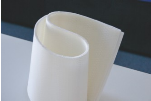
Wafer-thin, nearly transparent sheets from blocks of thermoplastics
