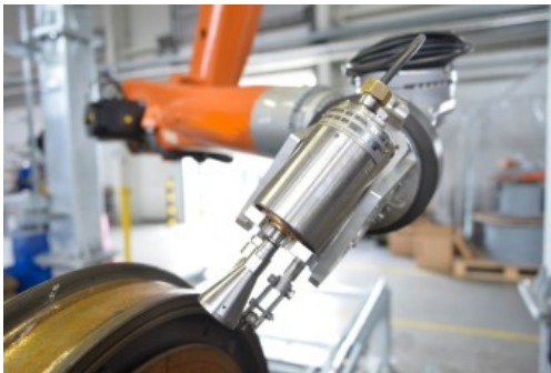
De-coating of a wheelset
