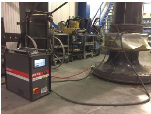
Betex MF Quick-Heater 3.0 in action
