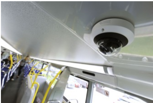
Mobile ME4 IR MicDome captures HD video, with IR LEDs and built-in mic to guard against moisture
