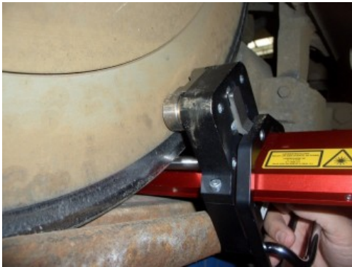
Wheel profile measuring device RPM BT
