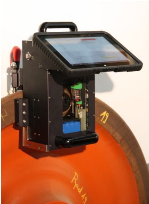
Determination of residual stresses in freight train wheels
