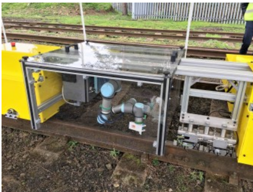
Inspection trolley with EMAT inspection and robot
