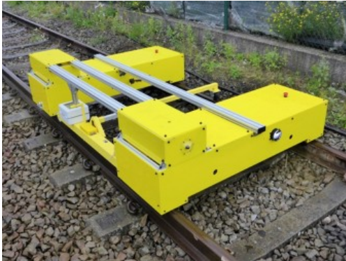
Motorized, autonomous inspection kart
