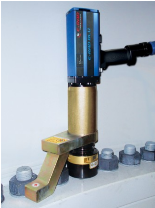
Electronic torque wrench E-RAD BLU
