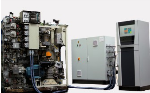
Test stand for air brake racks
