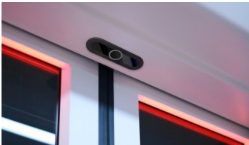
IRMA 6 – next generation of passenger counting; simulation of installation
