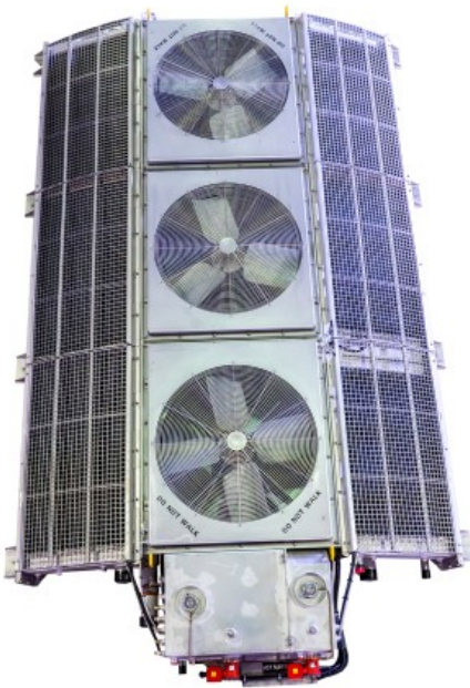
Radiator unit in VLocity DMU
