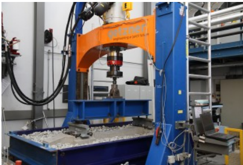
Under sleeper pads test confirms conformity to the new EN 16730
