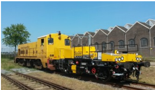
SIM14: Switch Inspection and Measurement vehicle
