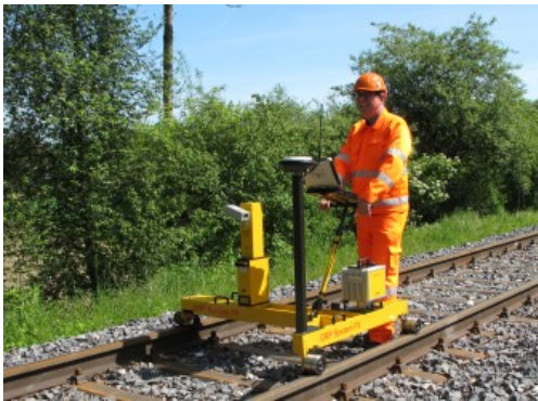
Amberg IMS 3000 with GNSS option for as-built track survey
