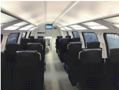
T5 tubular lights in the train
